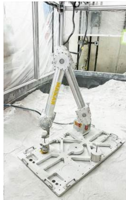
Figure 1: LUnA conducting functional demonstration during dust mitigation testing at the Lunar Testbed Facility, Colorado School of Mines
