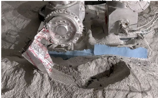
Figure 2: LUnA performing trench digging using the SAMPLR scoop at the Lunar Testbed Facility, Colorado School of Mines
